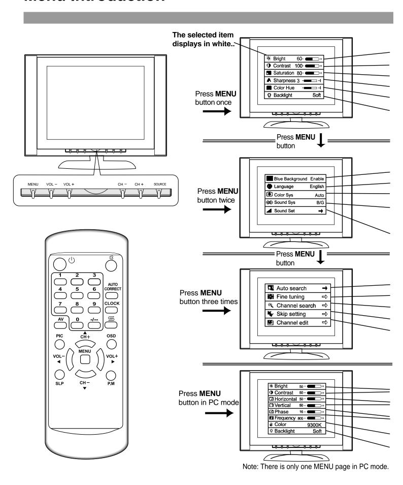
In **MENU** operations, the **CH+/-** buttons are used to select item upwards or downwards; the **VOL+/-** buttons are used to adjust or confirm selected item.
